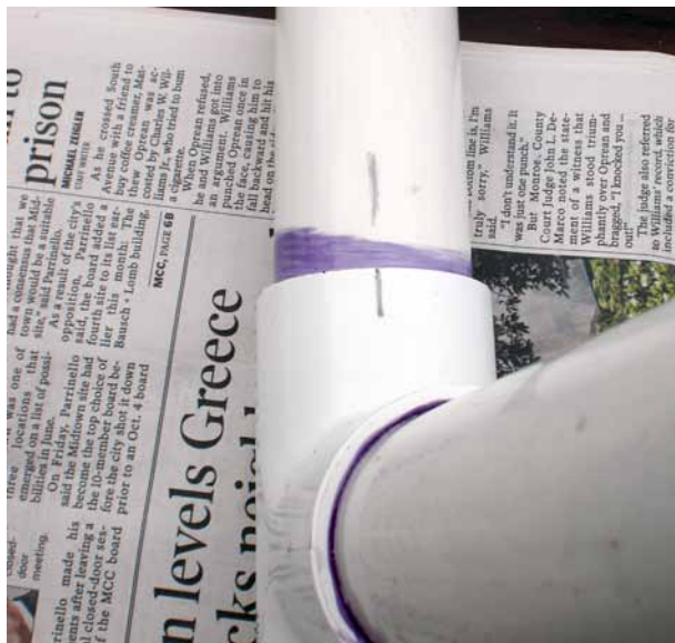
Figure 12: Make marks on the pipe and T when the angle is correct.
