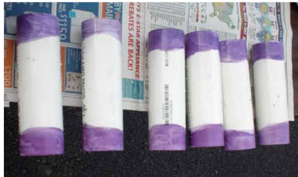
Figure 6: Pipes being primed. Hang them over the end of a table so the primer doesn't run.
