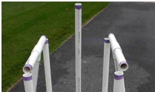
Figure 16: Braces attached to the two side diagonals.
