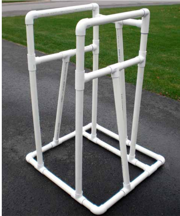
Figure 2: Redesigned dip stand with bracing.
