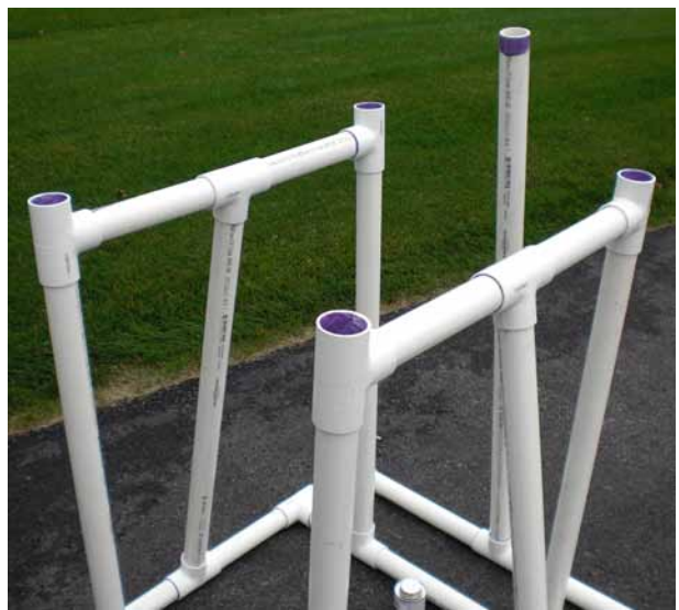
Figure 18: Diagonal braces locked into place.
