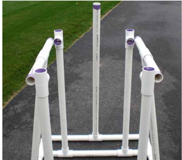
Figure 17: The T's attached to the uprights.
