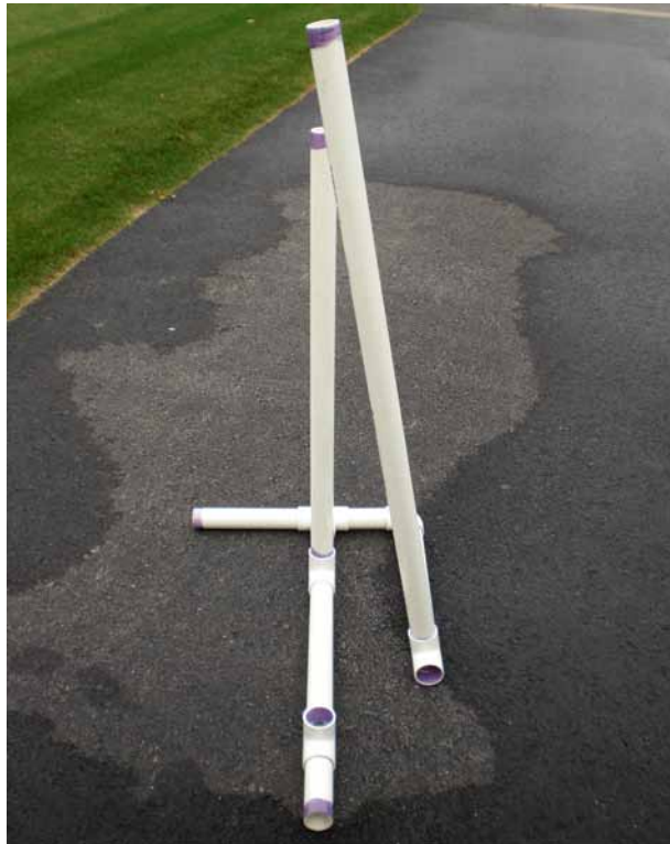
Figure 11: Line the diagonal pipe up with the tops of the uprights.
