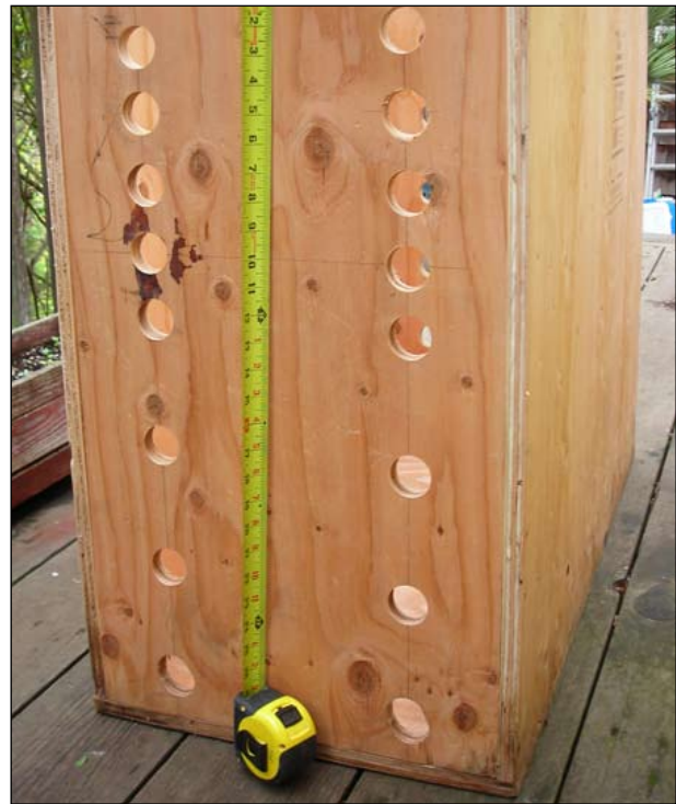
Figure 1: A series of holes allow an outer box to reach a height of 58 inches—high enough to satisfy even the elite skyloids at your box.
