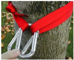
Once the anchors were set, we tied a figure eight knot and used a biner to attach the main line to the runner.
