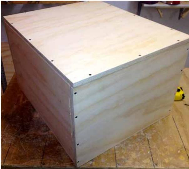
***When screwing the top down, use only one screw per side until you're sure the edges are lined up.***
