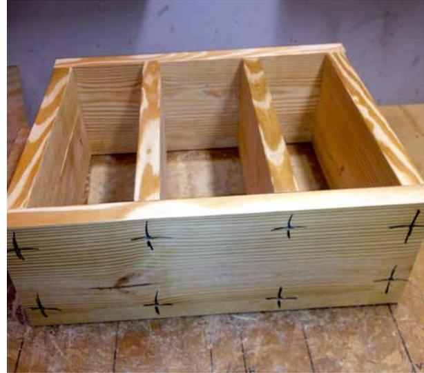
***Pre-drilling a few holes can make this step easier.***
