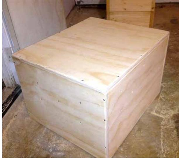
***Sanding the box and its edges is a nice touch that can save shins in the long run.***
