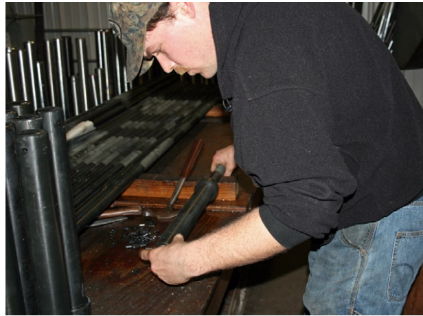
A sleeve is fitted to the bar shaft.
