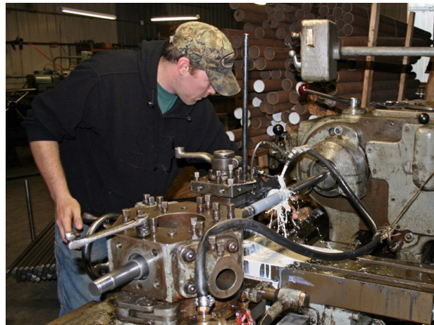
A bar shaft is turned down to size.
