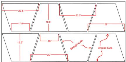
(left) a cardboard mockup helps make sure the box is the right size for your application. (right) how to make the most of your plywood.
